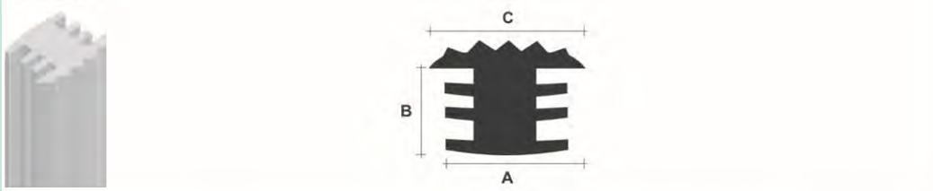
The image shows a 3D perspective view of a grey T-profile with two gripping fingers on the left and a black cross-section on the right. The cross-section has a top width labeled 'C', a bottom width labeled 'A', and a height labeled 'B'.
