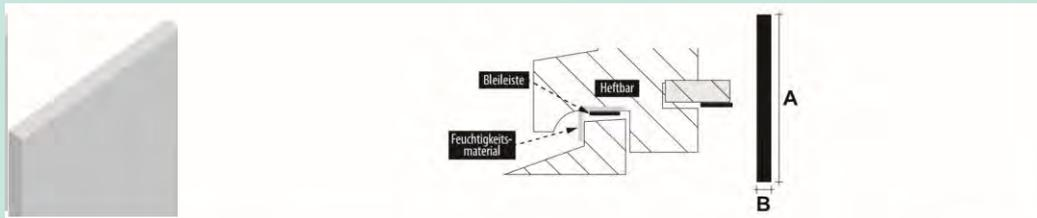
The image shows a 3D perspective view of a grey L-shaped profile on the left and a cross-section on the right. The cross-section shows the profile being attached to a surface with a 'Heftbar' (adhesive) and 'Feuchtigkeitsmaterial' (moisture material). The height of the profile is labeled 'A' and the thickness is labeled 'B'.
